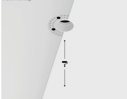
Push the lamp body upwards
